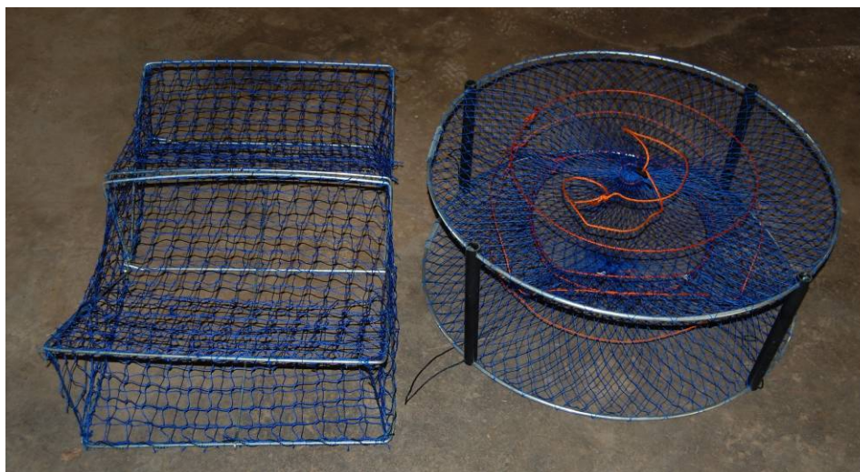
Figure 2.2. Two styles of collapsible polyethylene-mesh pots. The rectangular pot folds and locks in the centre of the longest axis (similar to a purse). The circular pot is held open by four grooved PVC uprights that, when disengaged from the top hoop, allow the pot to fold flat.
